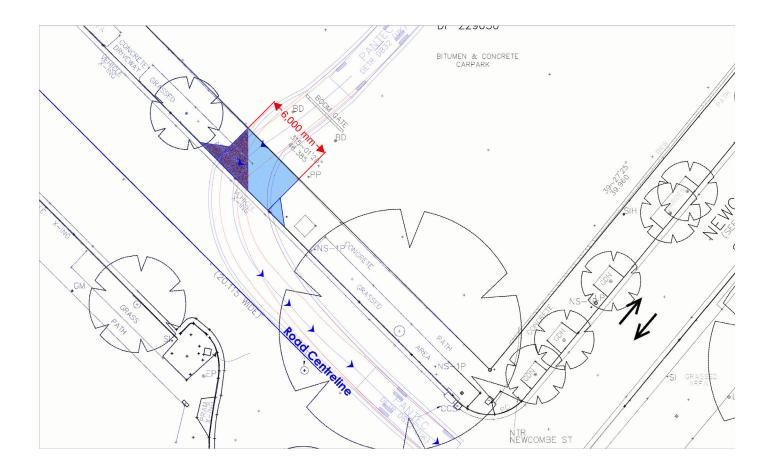
testing the different settings to gauge the difference in the resultant swept paths."
